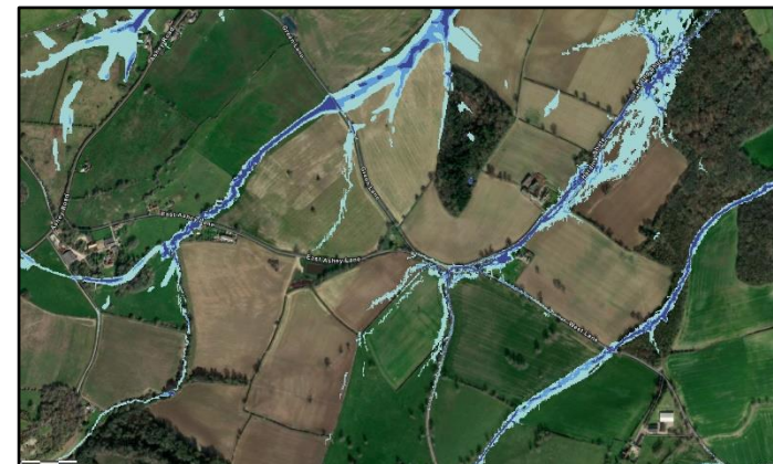
Figure 15. Risk of surface water flooding 15
